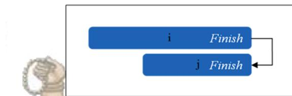
Gambar 2. 16 Ilustrasi Hubungan *Finish to Finish*
