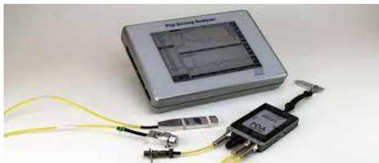
Gambar 2. 18 *Pile Driver Analyzer*
