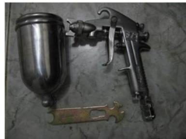
Gambar 1. Alat semprot (Spite) *airbrush*
