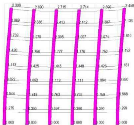
Gambar 2. 5 Deformasi as F tanpa construction stage analysis
