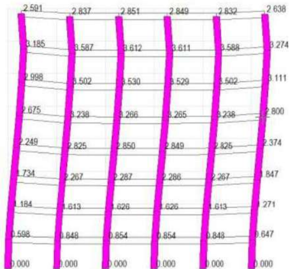
Gambar 2. 6 Deformasi as F dengan construction stage analysis
